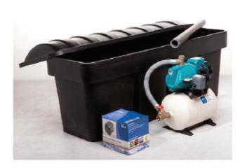
Aeration tanks gas off the rotten egg smell of hydrogen sulphide also allowing oxygen into the water improving precipitation of iron.
